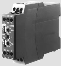
The S3UM voltage monitoring relay is used to monitor over and under-voltage and the phase sequence in 3-phase supplies.
